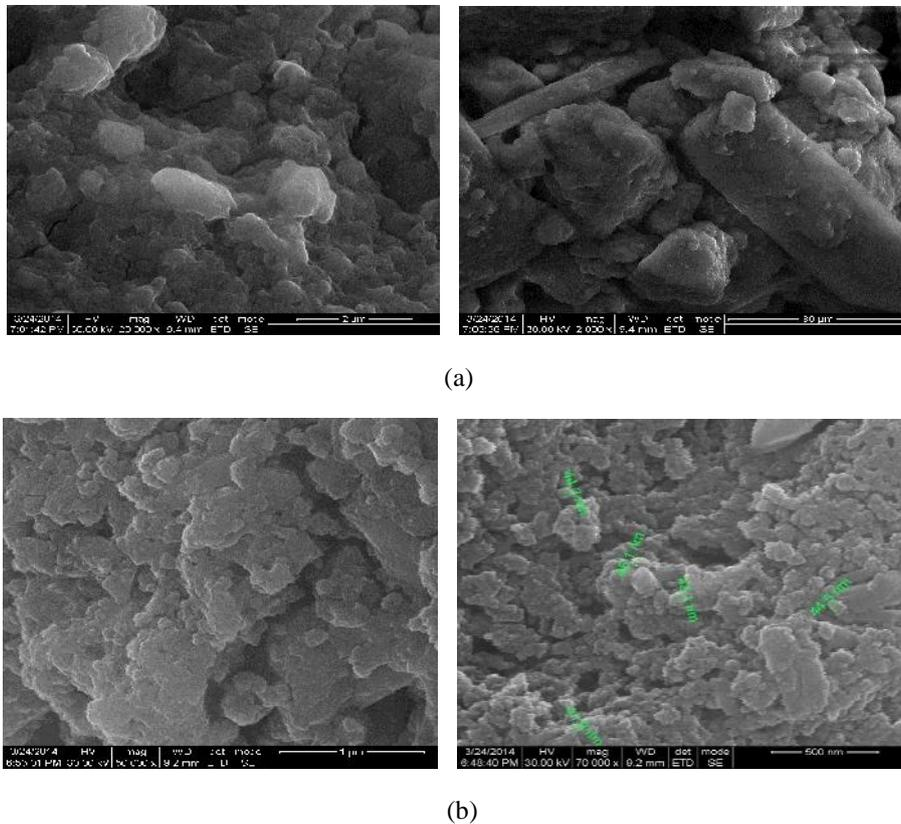
Figure (3) SEM images of (a) CdZnBaFe<sub>2</sub>O<sub>4</sub> for as 2 & 30 μm (b) CdZnSrFe<sub>2</sub>O<sub>4</sub> for as 1 μm & 500nm
