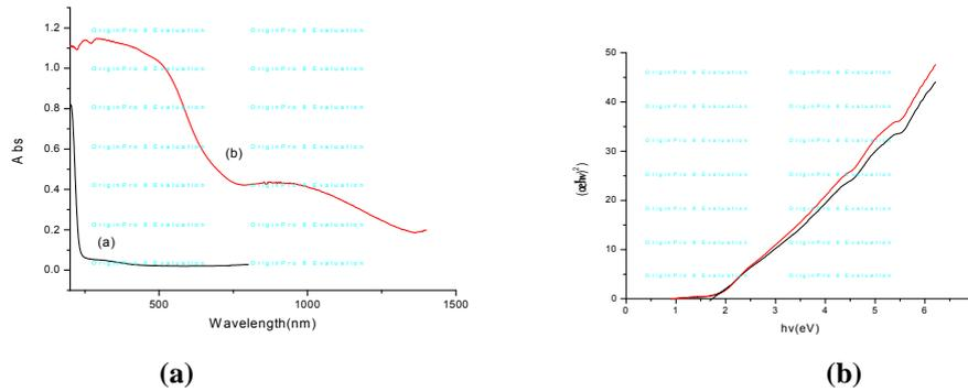
Figure 2.(a)Absorbance spectra of CdZnBaFe<sub>2</sub>O<sub>4</sub> & CdZnSrFe<sub>2</sub>O<sub>4</sub>, (b) Plot of  $(\alpha h\nu)^2$  vs  $h\nu$  for CdZnBaFe<sub>2</sub>O<sub>4</sub> and CdZnSrFe<sub>2</sub>O<sub>4</sub>
