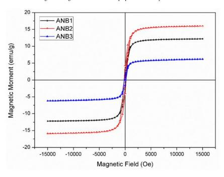
Figure 5: Magnetization curve of annealed Ni-B alloy
