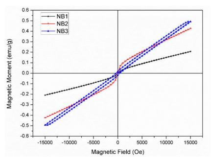
Figure 4: Magnetization curve of as prepared Ni-B alloy
