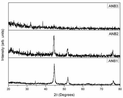
Figure 2: XRD pattern of annealed Ni-B alloy
