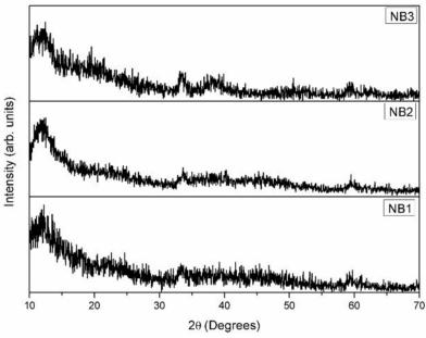
Figure 1: XRD pattern of as prepared Ni-B alloy
