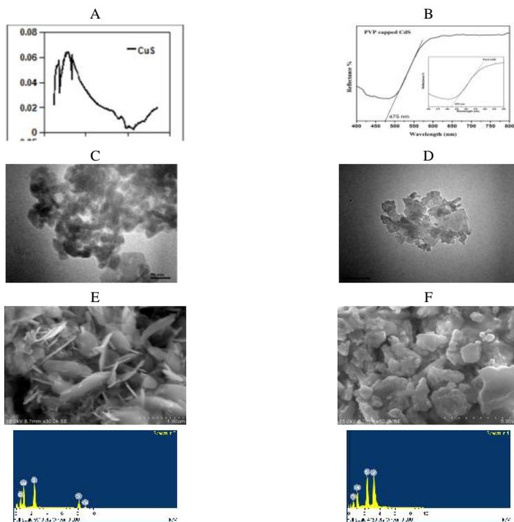
Fig.1 UV-DRS(A, B), HRTEM photos (C, D) and FESEM with EDX (E, F) of CuS NPs and CdS NPs in the synthesized samples
