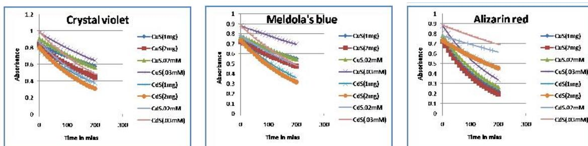
Fig.2 The absorbance variation with time plots of CV, MLB, AR dyes in the presence of CuS NPs and CdS NPs
