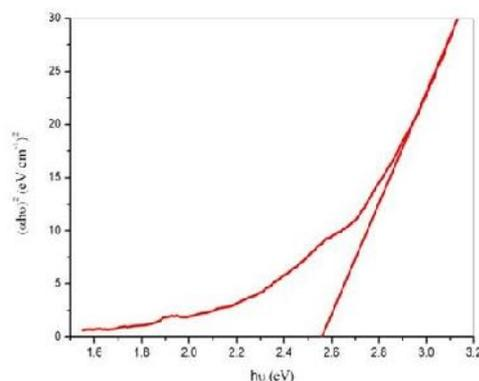
Fig. 4 Bandgap of CdO microplates
