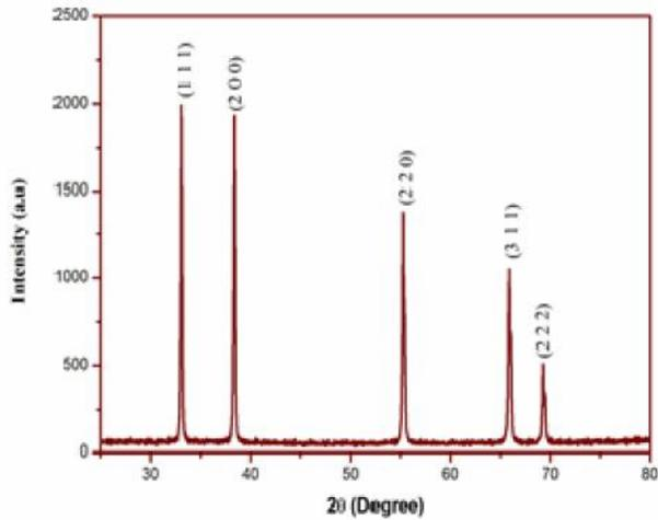
Fig.1 XRD pattern of CdO microplates
