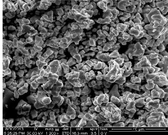
Fig.2 SEM image of CdO microplates
