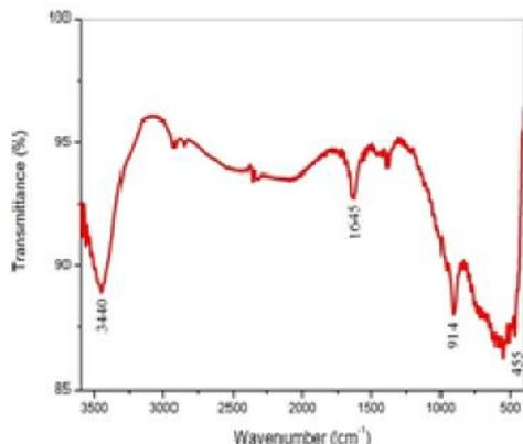
Fig. 3 FT-IR spectra of CdO microplates
